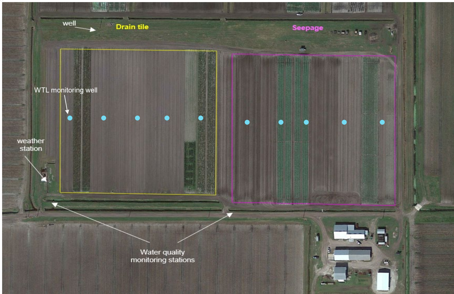
Figure. Aerial image of UF/IFAS Hastings Agricultural Extension Center, in Hastings, FL. The yellow polygon indicates drain tile area and the pink polygon indicates the seepage irrigated area. Arrows indicate water quality monitoring stations and weather station. White polygons indicate a test bed with N and P treatments conducted during spring potato season. Blue dots indicates the water table level (WTL) monitoring wells.
